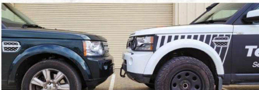
Standard height vehicle vs vehicle fitted with conversion kit TF266
